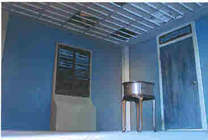
1 Two digital flats simulating plaster walls in conjunction with real table, window, and door props create a virtual room.
