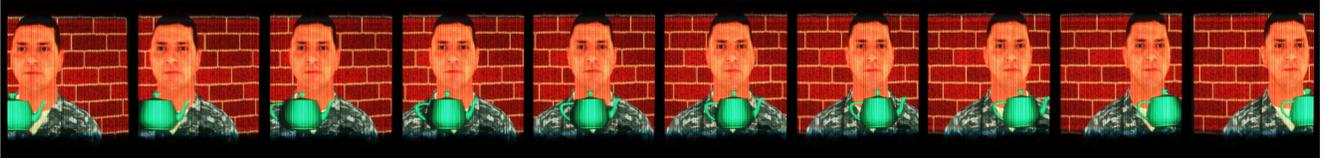
Figure 6. Long-exposure photographs of the display prototype from different camera positions with 4mm spacing between projector positions. Neighboring images can be seen in 3D through cross-fusion. Horizontal parallax is visible between teapot, human, and wall at different depths; the deep depth of field allows all three objects to remain in focus with smooth motion parallax (see accompanying video).
