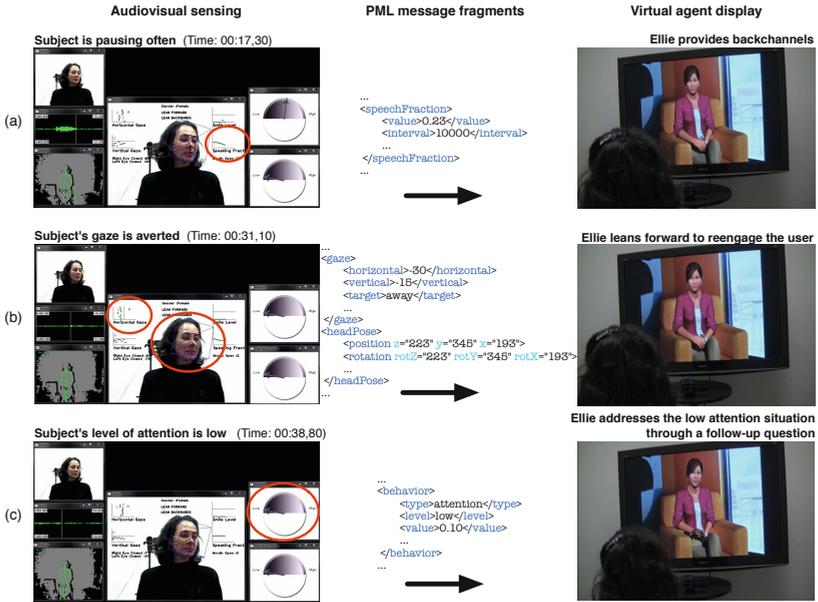
**Fig. 3.** Display of multimodal nonverbal behavior analysis (i.e. Multisense; left column) shown with corresponding PML message fragments (middle column) and virtual agent reactions (right column). Times indicate position in supplementary video.
