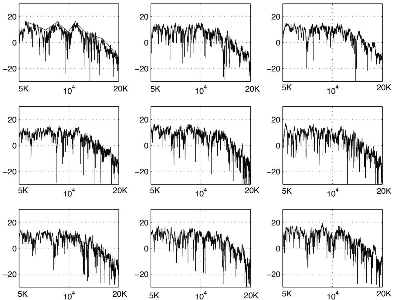
Fig. 2: Magnitude Responses for the nine locations in the 5-20 kHz range. An approximated piecewise linear envelope of the resonant peaks is shown for the response in the first row and first column.
