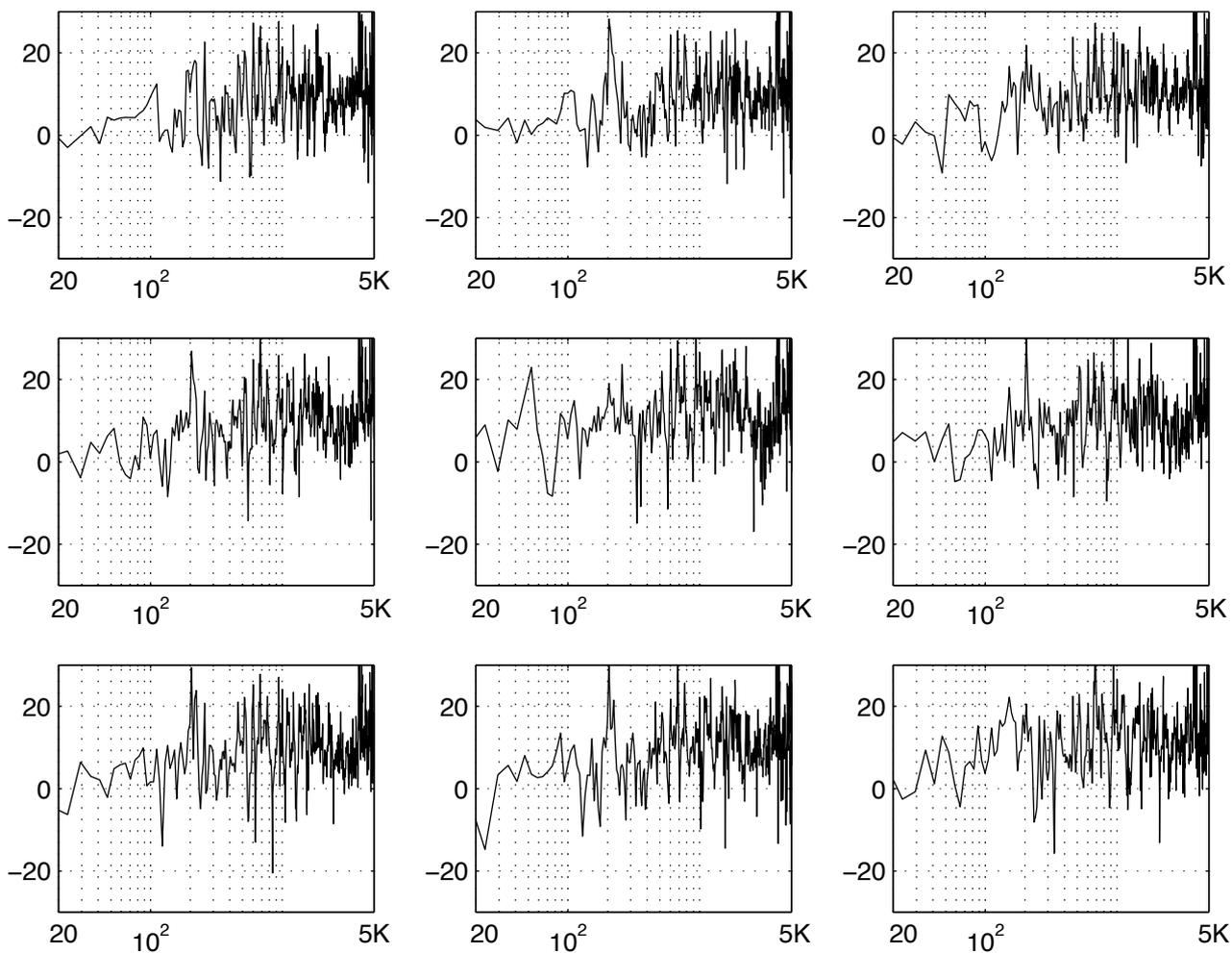
Fig. 3: Deviation from flatness of the magnitude responses for the nine locations, of Fig. 1, in the 20 Hz-5 kHz range using spatial averaging based equalization.
