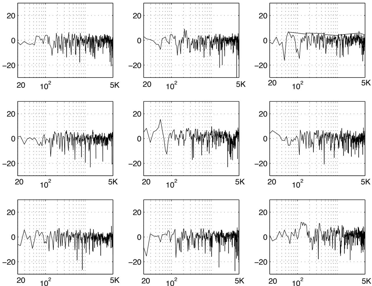
Fig. 5: Deviation from flatness of the magnitude responses for the nine locations, of Fig. 1, in the 20 Hz-5 kHz range using the proposed fuzzy c-means clustering approach. An approximated piecewise linear envelope of the resonant peaks is shown for the response in the first row and third column.
