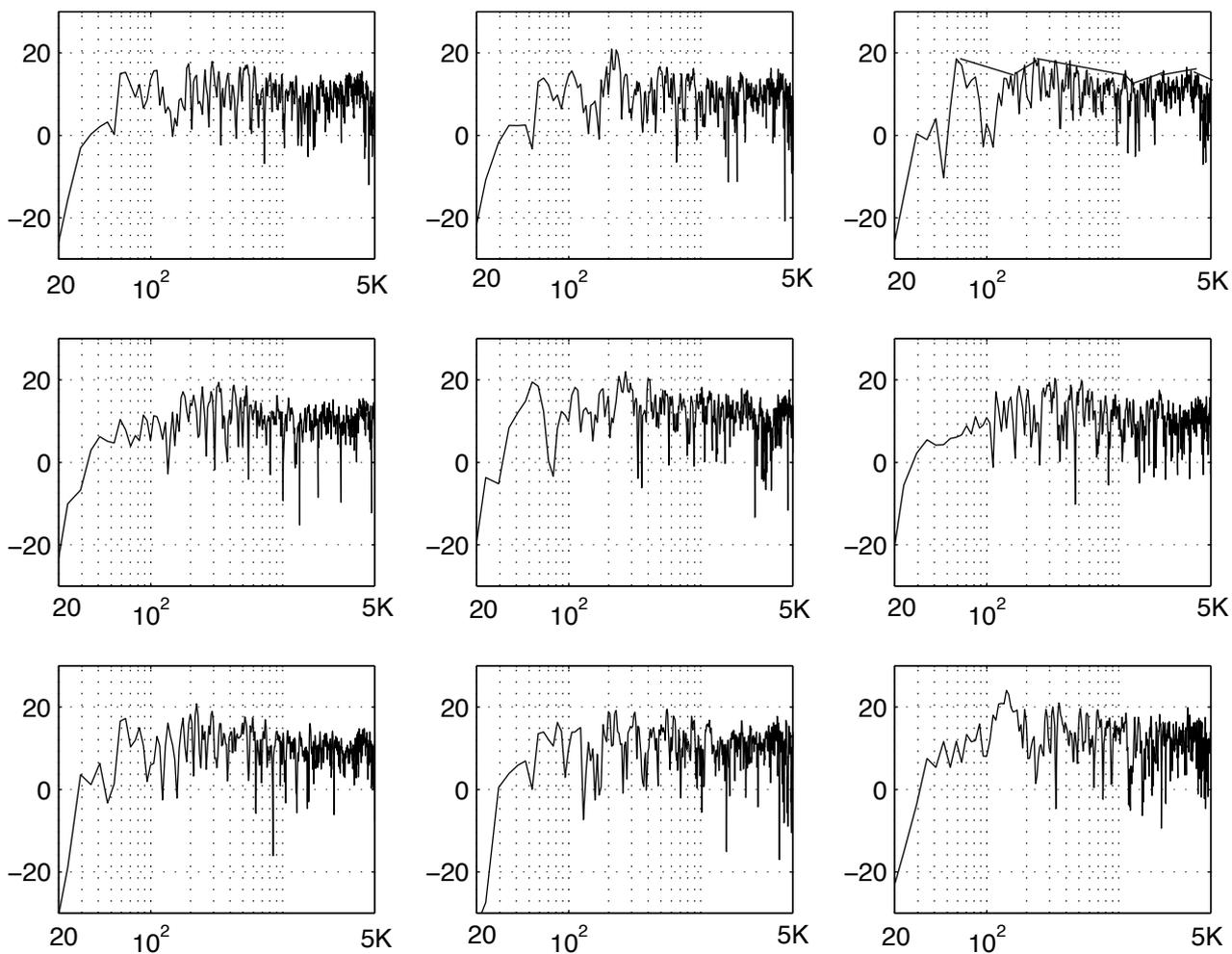
Fig. 1: Magnitude Responses for the nine locations in the 20 Hz-5 kHz range. An approximated piecewise linear envelope of the resonant peaks is shown for the response in the first row and third column.
