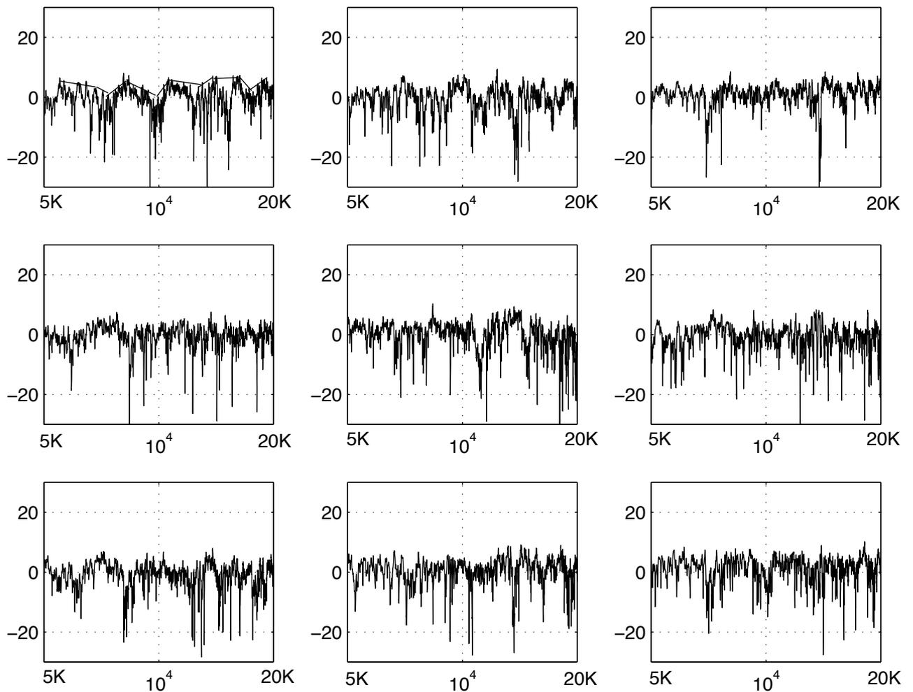
Fig. 6: Deviation from flatness of the magnitude responses for the nine locations, of Fig. 1, in the 5 kHz-20 kHz range using the proposed fuzzy c-means clustering based equalization. An approximated piecewise linear envelope of the resonant peaks is shown for the response in the first row and first column.
