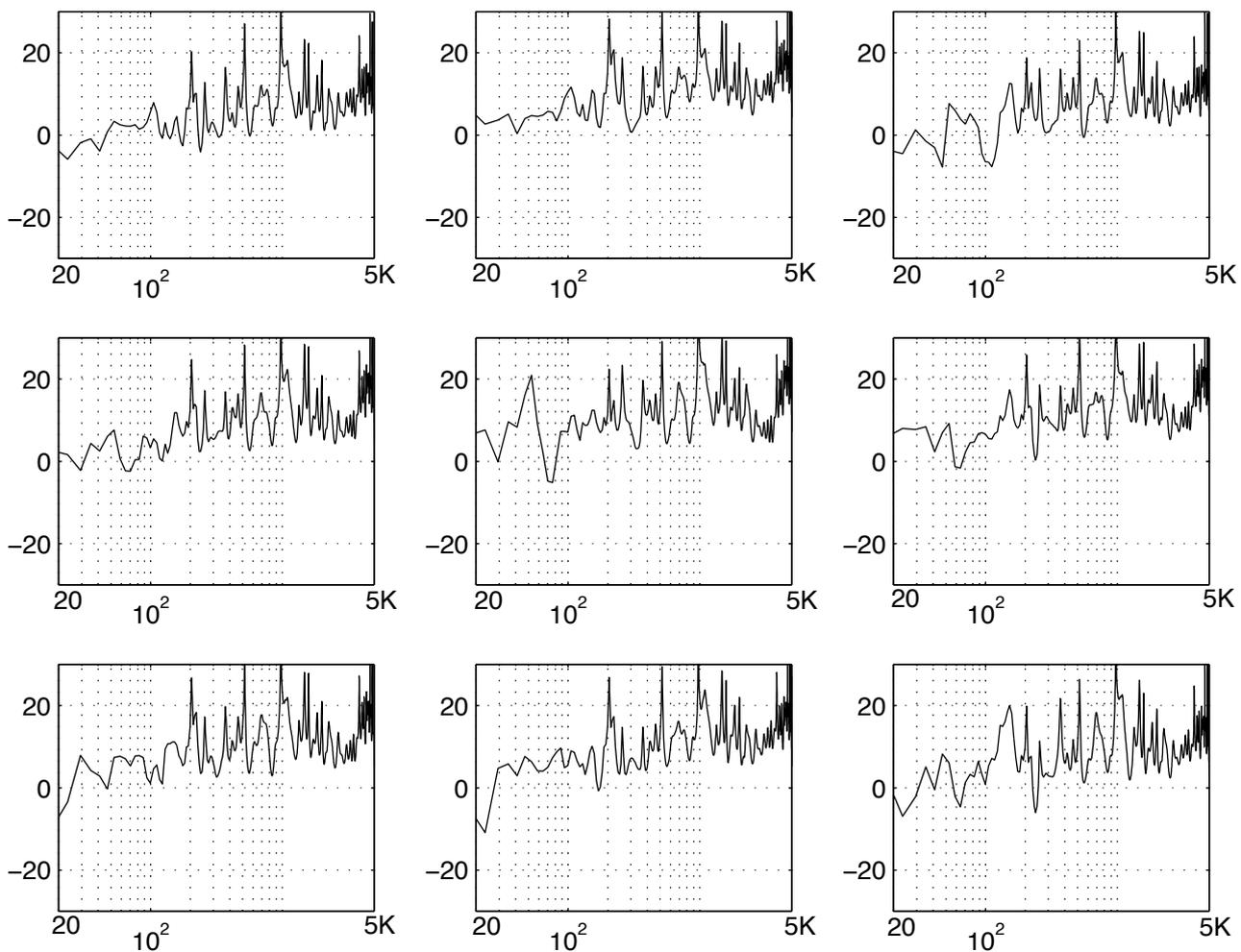
Fig. 8: Deviation from flatness of the magnitude responses for the nine locations, of Fig. 7, in the 20 Hz-5 kHz range using spatial averaging based equalization.
