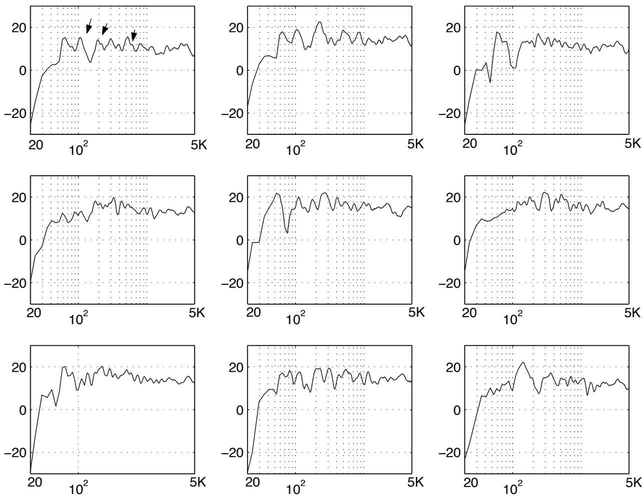
Fig. 7: Smoothed magnitude responses of Fig. 1. An approximated piecewise linear envelope of the resonant peaks is shown for the response in the first row and first column.
