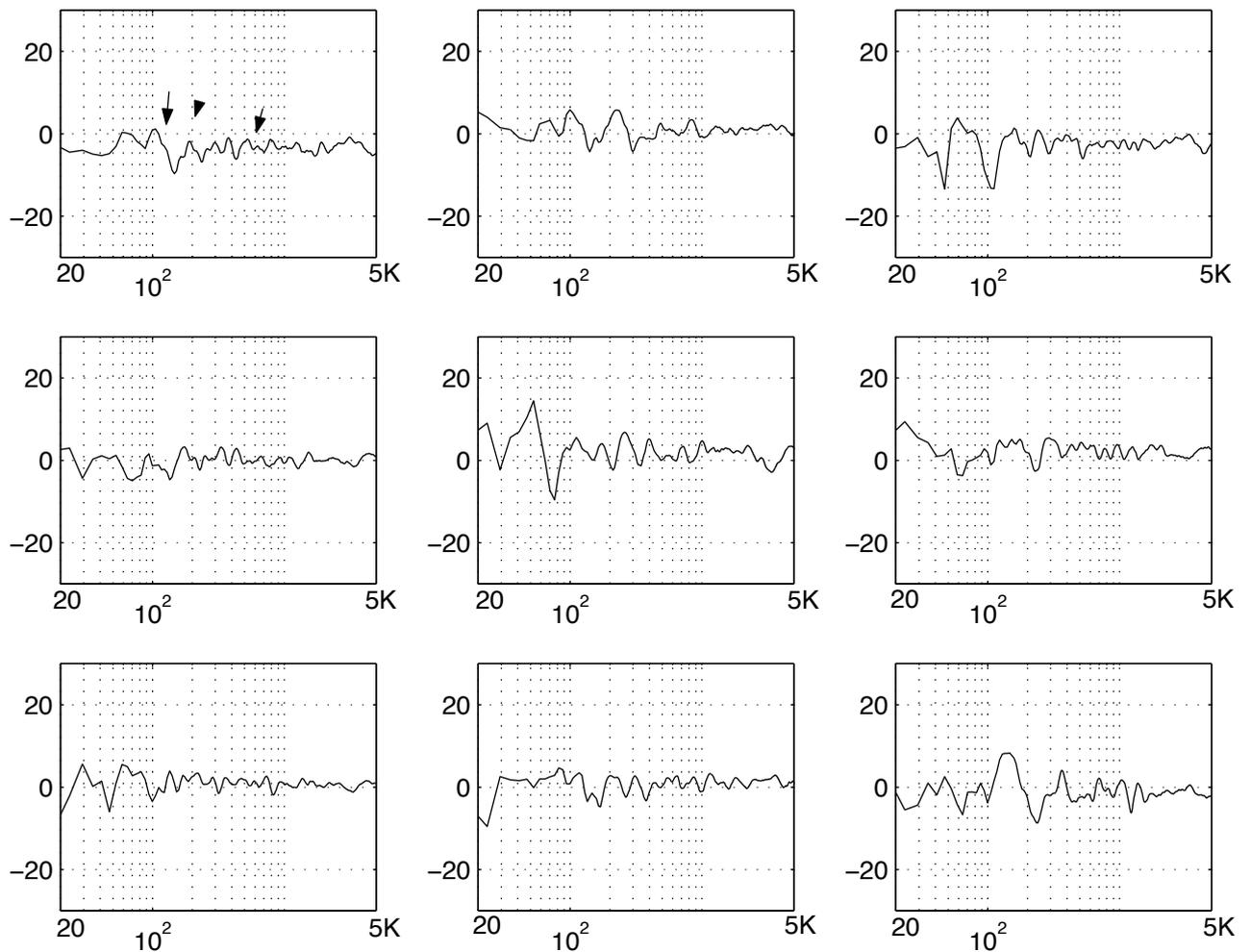
Fig. 9: Deviation from flatness of the magnitude responses for the nine locations, of Fig. 7, in the 20 Hz-5 kHz range using using the proposed fuzzy c-means clustering based equalization. An approximated piecewise linear envelope of the resonant peaks is shown for the response in the first row and first column.
