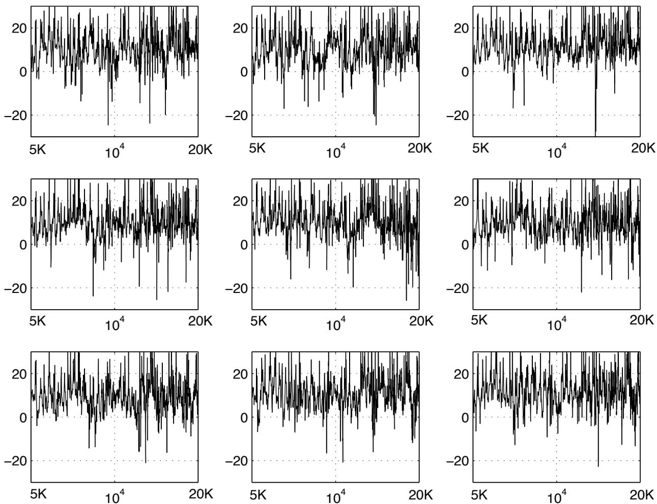
Fig. 4: Deviation from flatness of the magnitude responses for the nine locations, of Fig. 2, in the 5 kHz-20 kHz range using spatial averaging based equalization.
