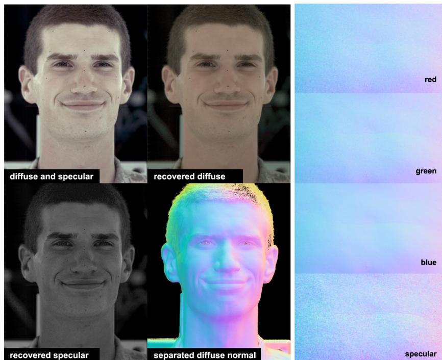
**Figure 3: Color space separation of diffuse and specular components of the acquired images. Clockwise from top left: captured albedo under uniform spherical illumination, separated diffuse albedo, separated diffuse normal, separated specular albedo. Right column: separated (red, green and blue) diffuse and specular normals.**
