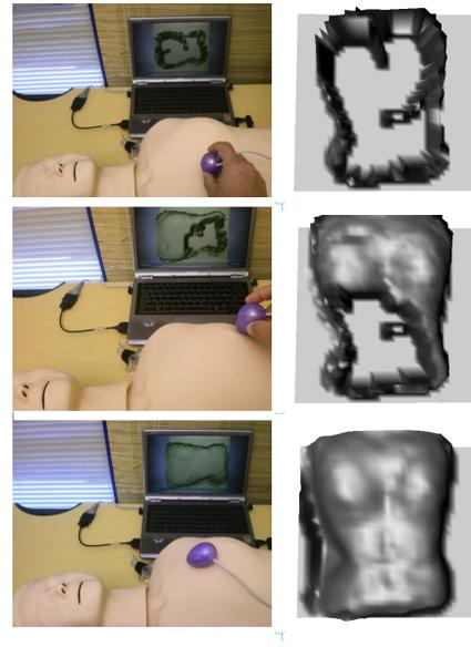
Figure 3: Scanning Anne torso: initial contour, intermediate, final mesh. Grid: 40 x 40 cm, 40 x 40 points. Scanning time: 8 minutes. The 3D snapshots are shown "as is", without retouching.
