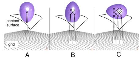
Figure 4: A plastic eggshell provides three intuitive scanning positions: (A) contact with the pointed end moves one vertex; (B) the obtuse end moves the vertex and its closest neighbors (5 points per move); (C) contact with the elongated area makes the system to iterate on vertex neighbors twice (13 points per move).
