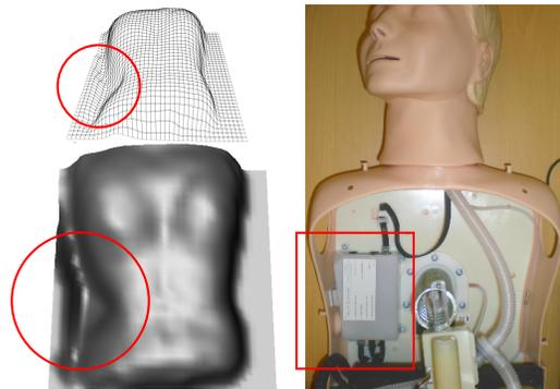
Figure 5: Distorted surface area, denoted by a circle. A 'postmortem' examination revealed that Anne was engineered asymmetrically: a metal switchbox installed in her upper right abdominal area, caused distortions in the magnetic field. Embedding these distortions into the model effectively cancels their effect during model use.
