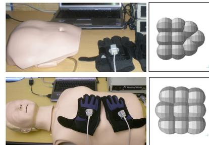
Figure 1: Augmented manikins. The system components: manikin objects from Laerdal [3], Flock of Birds tracking system from Ascension [4], a laptop PC (1.86 GHz CPU, 1G RAM, Linux OS).
