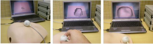
Figure 2: Scanning SimMan's abdomen module, left to right: sensor alignment; scanning in progress; completed mesh. Grid size 40 x 40 cm, 20 x 20 points. Scanning time: less than 2 minutes.
