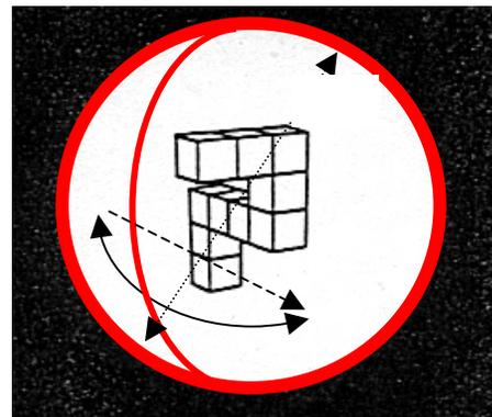
**Figure 4:** The Arcball interface interaction method (Shoemake, 1992). The dotted line is the dragging action on the 2D projection display surface using the mouse and the solid line represents the rotation direction around the axis of the red sphere overlaid around the object.
