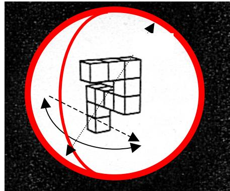
**Figure 4:** The Arcball interface interaction method (Shoemake, 1992). The dotted line is the dragging action on the 2D projection display surface using the mouse and the solid line represents the rotation direction around the axis of the red sphere overlaid around the object.
