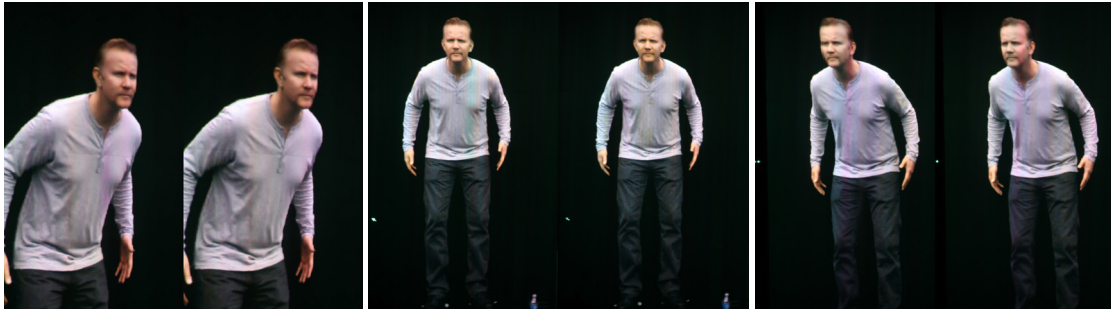
Figure 1: Three stereo photographs of Morgan Spurlock shown on the automultiscopic projector array. The display can be seen by multiple viewers over a 135° field of view without the need for special glasses. The images are left-right reversed for cross-fused stereo viewing.
