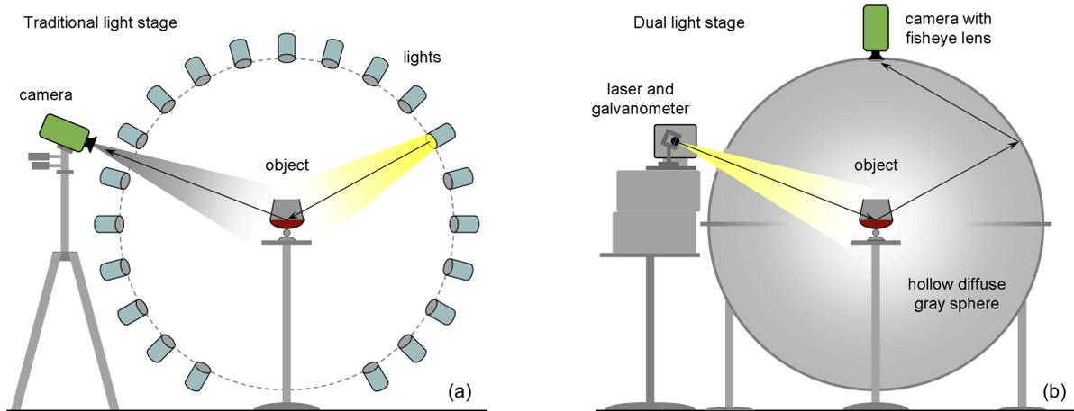
**Figure 1:** (a) A traditional light stage, where an object is progressively photographed as illuminated by a number of lighting directions. (b) A dual light stage, where a laser is scanned across the object and the scattered light forms images on the inside of a diffuse sphere. The reflectance function images are recorded by a camera with a fisheye lens that views the entire sphere.
