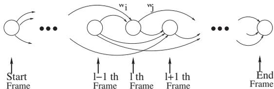
Fig. 2. A typical word lattice in ASR.
