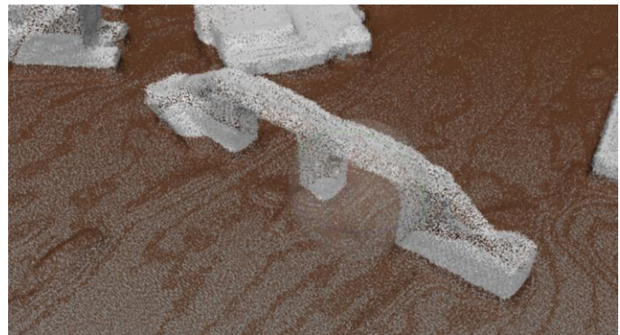
Figure 4. The pedestrian overpass and terrain, with ground (brown) and structures (white) classified.
