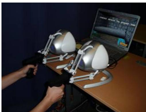
**Figure 3** Two Novint Falcon devices yoked together with a screen shot of the bimanual task
