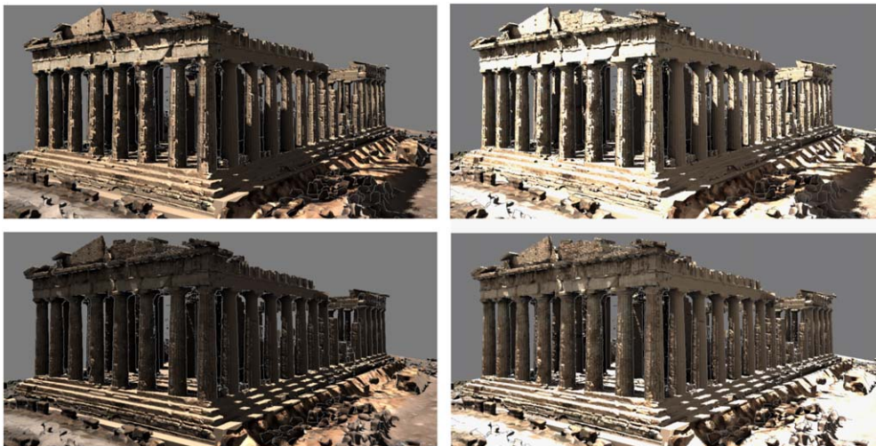
Fig. 2. Examples of realtime shading: note how the shadows moves precisely over the geometry (top-left and bottom-left images) and how the HDR lighting calculation allows to adjust the exposure to better perceive details (images on the right) which are under shadows in the images on the left.
