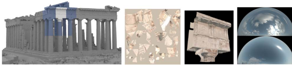
Fig. 1. Available data. The 3D model of the Parthenon building, acquired with TOF scanning and divided in multiple chunks (one of these chunks is rendered in white); the texture atlas used for the highlighted chunk, which encodes the recovered surface albedo, and the texture-mapped chunk; finally, HDR images of the sky dome.
