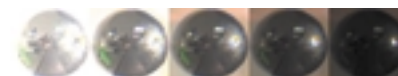
Figure 3. Five exposures of a high dynamic range image captured in a single frame.
