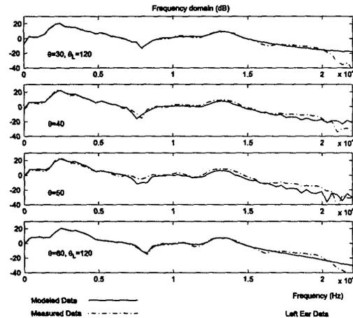
Figure 7: Frequency domain of measured and simulated impulse responses for a model created with a  $30^\circ$  resolution.  $\theta = 40^\circ$  and  $\theta = 50^\circ$  were not used for the creation of the model
