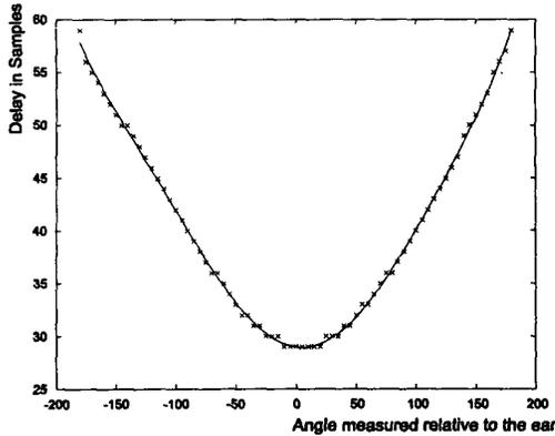
Figure 2: Extracted delay and sixth order polynomial fit.
